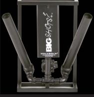
psi using an air compressor. The solenoid valve is actuated by electronic input from a 110 VAC power source. The Big Shots® can be easily modified to use a 220 VAC, a 24 VDC or a 12 VDC power source. The solenoid actuation requires approximately 20 watts each. The Big Shots® can be operated from a lighting board on a non-dim circuit.
